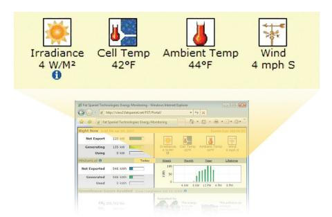
Our Full Weather Station enables you to see irradiance, cell temperature, air temperature, wind speed and wind direction on your personalized view.
